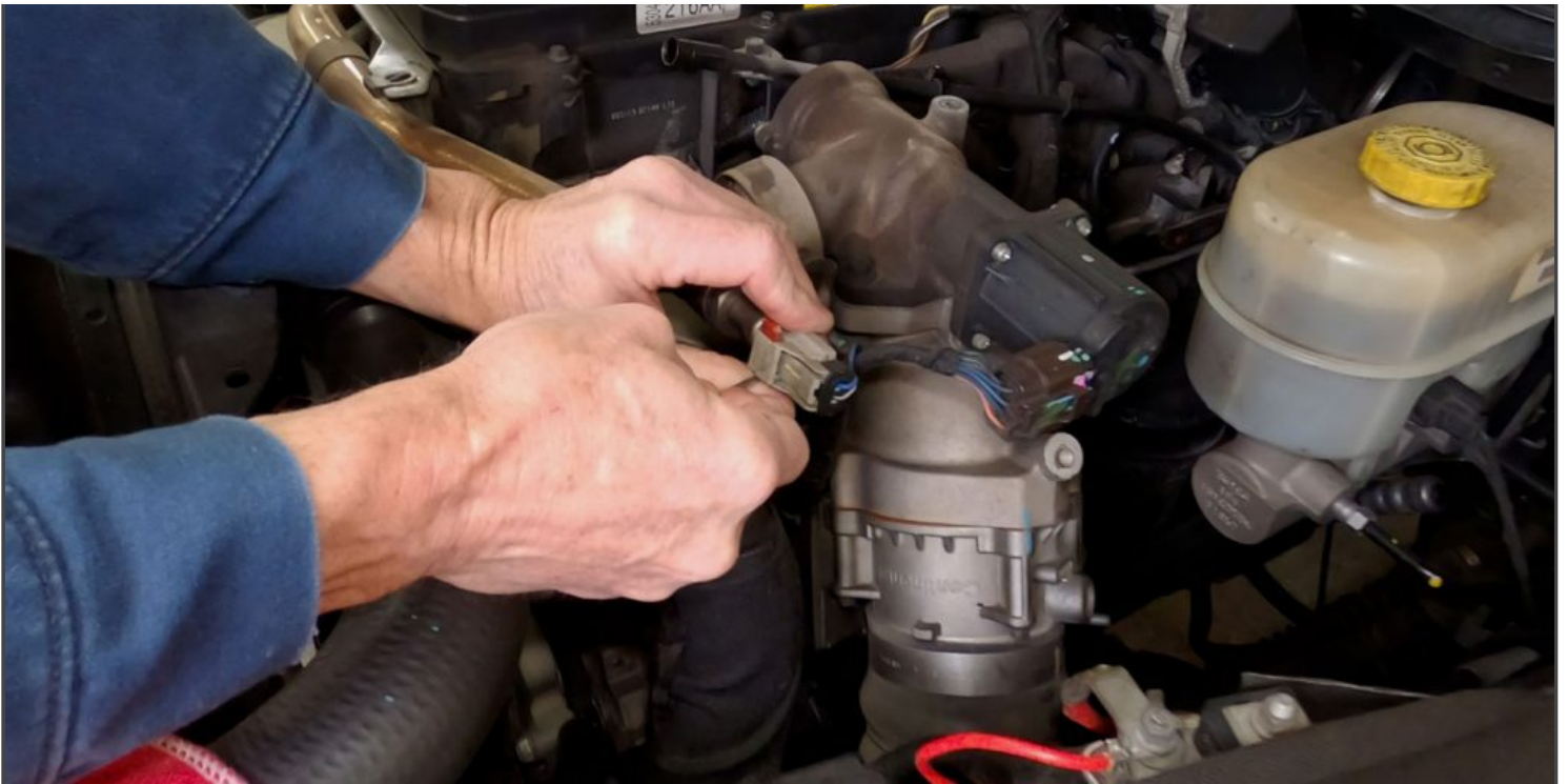
Forward EGR Temperature Sensor Location. If sensor is mounted to rear of Intake Elbow, refer to Step 6a
