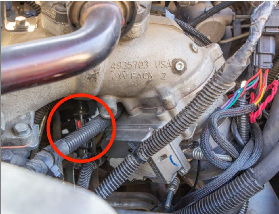
Location of connector for rear intake elbow mounted thermocouple.
