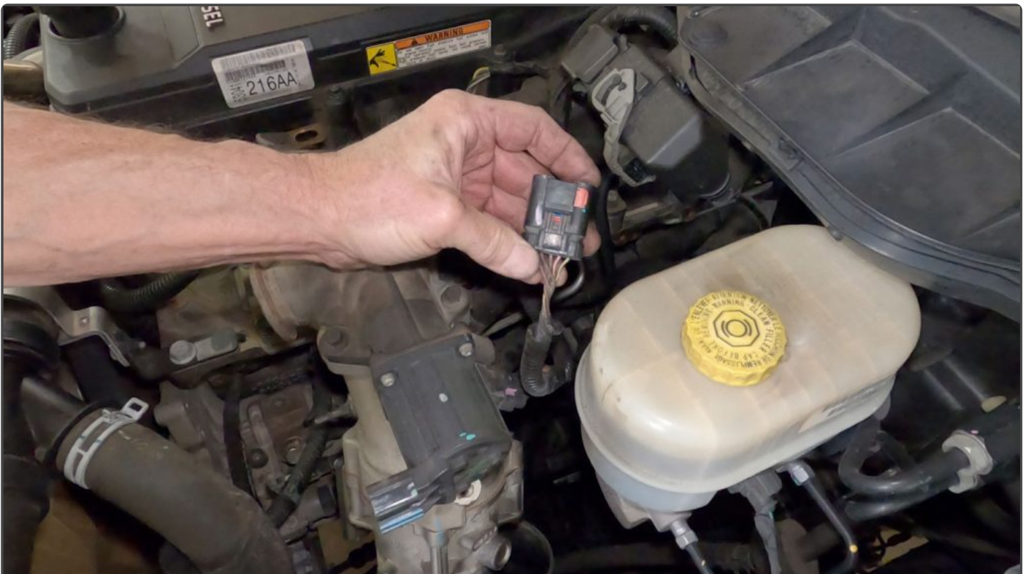
MAP Sensor and throttle body connector location.
